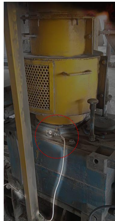
A Air Classifier/Separator With the Piezoelectric Uniaxial sensor
